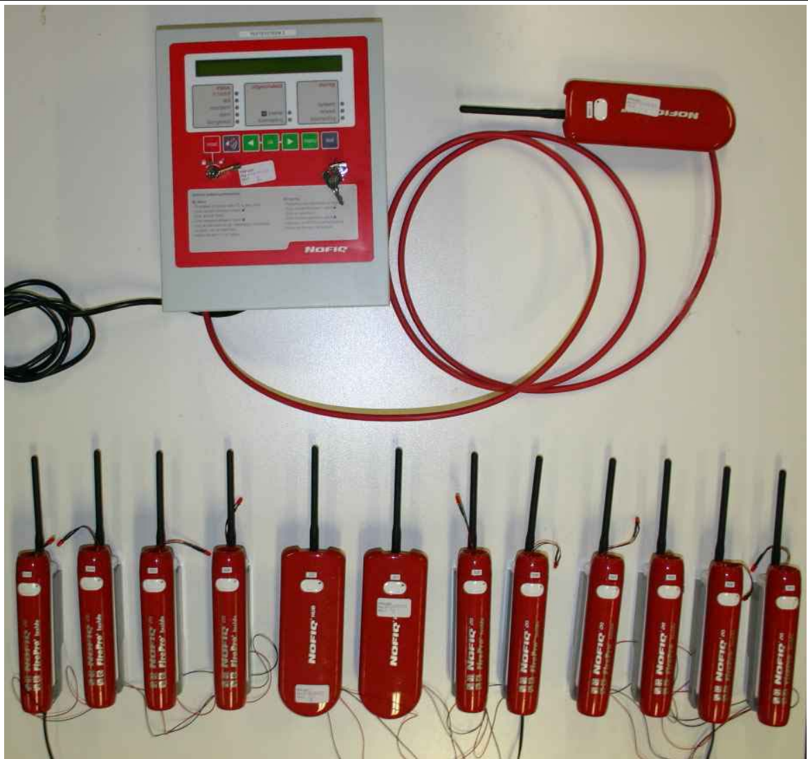
Overview of the system, Base with base-hub on top, below, FE's and Hubs
