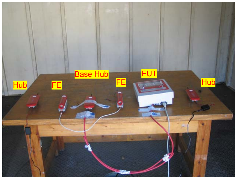
Photo 1. Total set-up of the EUT during testing, including Base Hub, Hub's and FE's
